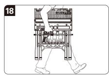
To carry Pegasus safely, only transport when folded, hold the table vertically and carry close to the body. (Fig. 18)
