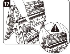
To fold Pegasus for storage: • Press both latches and collapse the table. (Fig. 16) • Lift the tool tray in the centre to allow the legs to fold. (Fig. 17) WARNING: Keep fingers away from moving joints to avoid pinching.
