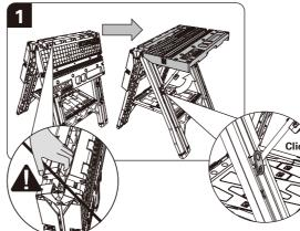
To use Pegasus as a work bench, open the legs fully and pull the table upward until latches "click" into place.(Fig. 1)
