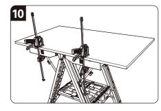
Quick clamps can be used independently if desired. (Fig. 10)
