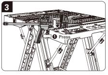
Align the Quick Clamps with the slot and insert it fully. Grip the Quick Clamps handle and put it into the groove as shown. Once the clamps are seated, release the handle. (Fig. 2-4)
